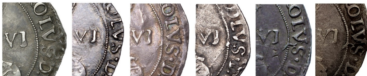
Figure 3: The progression of the die crack on Ob B. The left-hand image is taken from a B-5 coin before the crack appeared (all images except rightmost two are © Noonans Mayfair Ltd)
