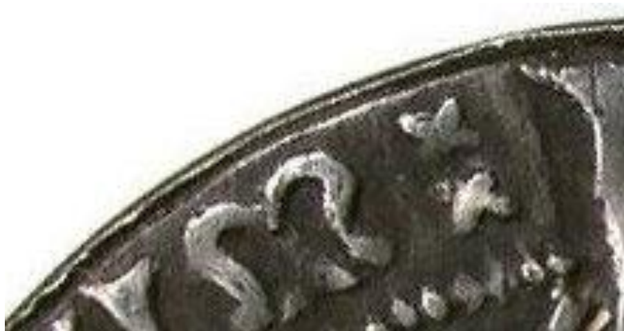
Fig. 4. Tell-tale edge feature from casting
