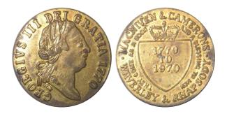
Metals: Cu 69.7%, Zn 30.2%, Sn 0.033%, Fe 0.018% - C260 Cartridge Brass.
