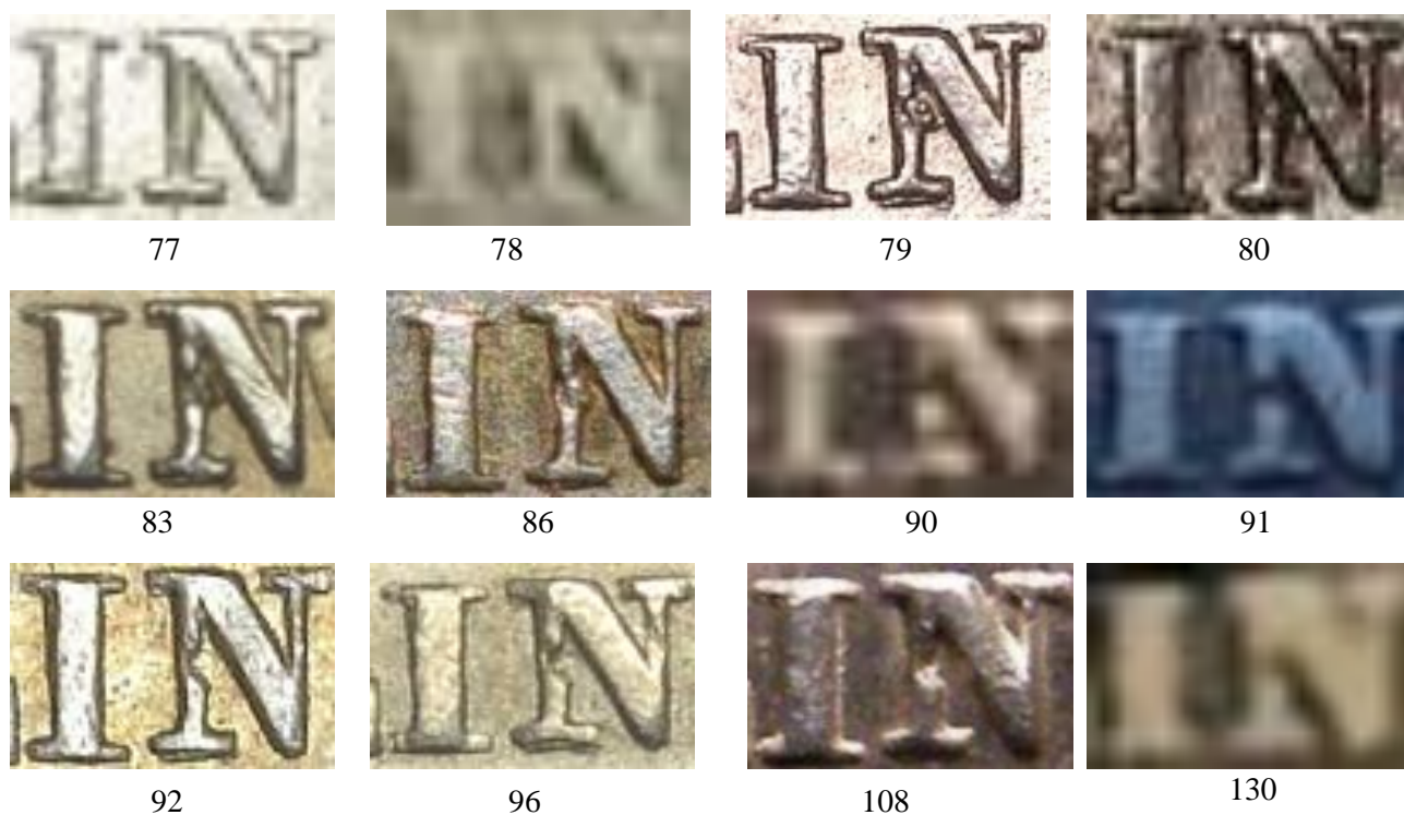
Fig. 1. First appearance and development of die flaw in N of SHILLING for 1865.
